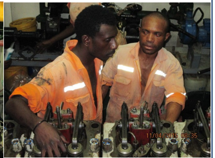
Mell Manuai and David Jujembo overhauling a cylinder head.
